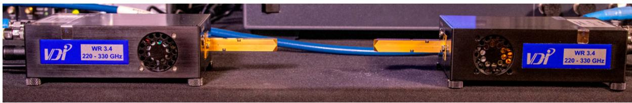
**Figure 4.** Over-the-air (OTA) Test Case Using Diagonal Horn Antennas
