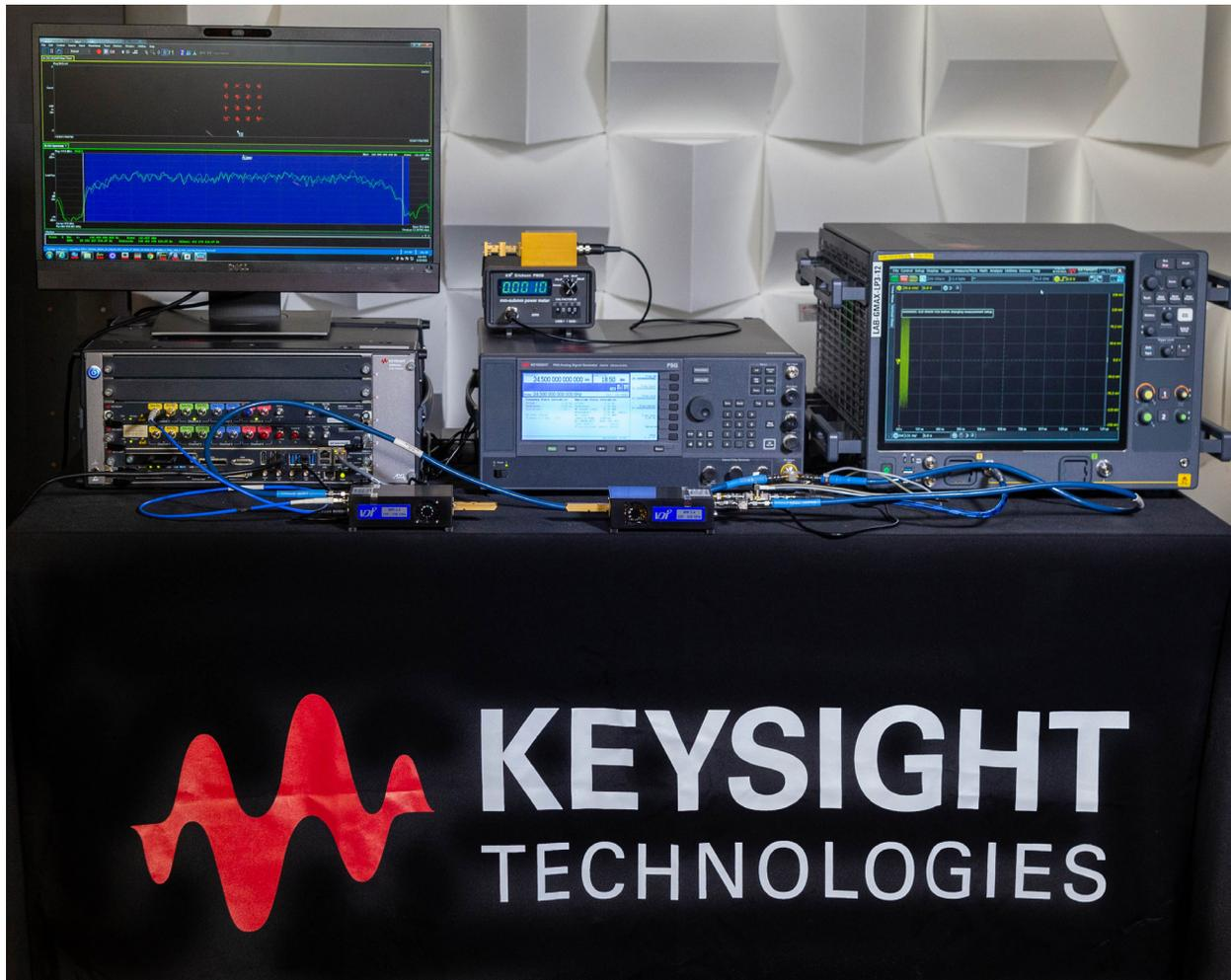
Figure 2. Sub-THz Testbed for H-Band, 220-330 GHz
