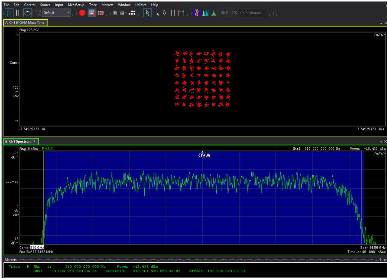
**Figure 5.** Over-the-air (OTA) Measurement Results at 310 GHz for the 30 GHz Bandwidth Test Case
