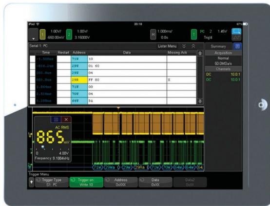
Figure 37. Tablet virtual front panel control.
