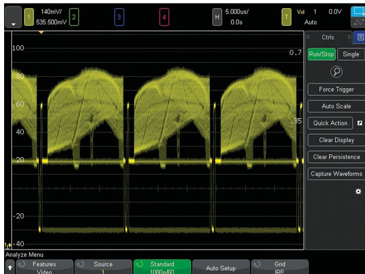
Figure 27. Triggering on 1080p HDTV signal analysis.
