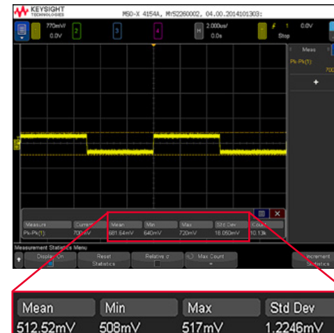
100 KHz clock signal
