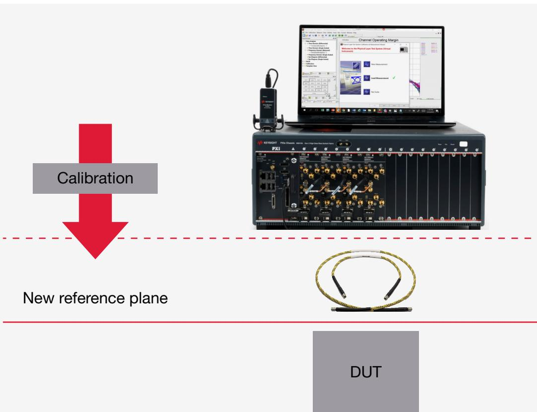
Figure 4: Calibration test setup with reference plane
