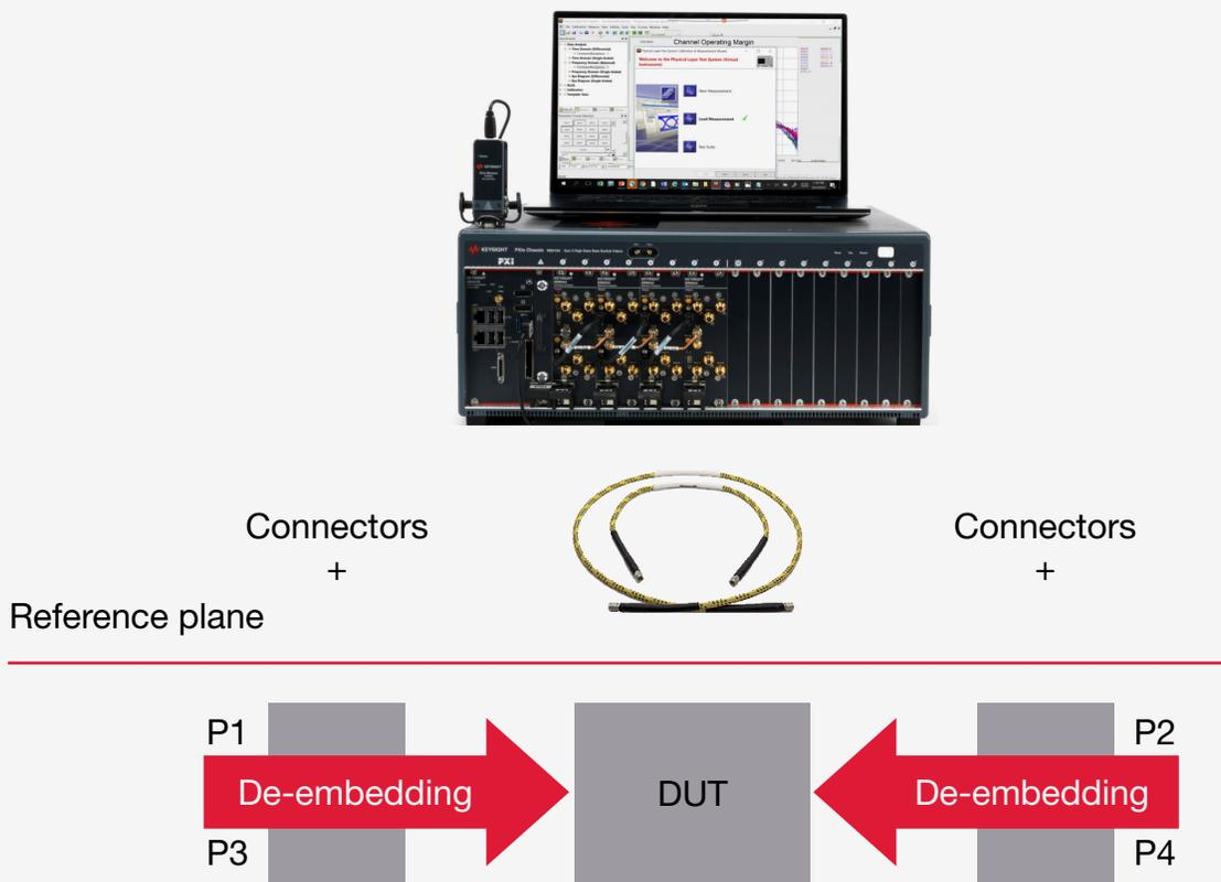
Figure 5: De-embedding test setup with reference plane
