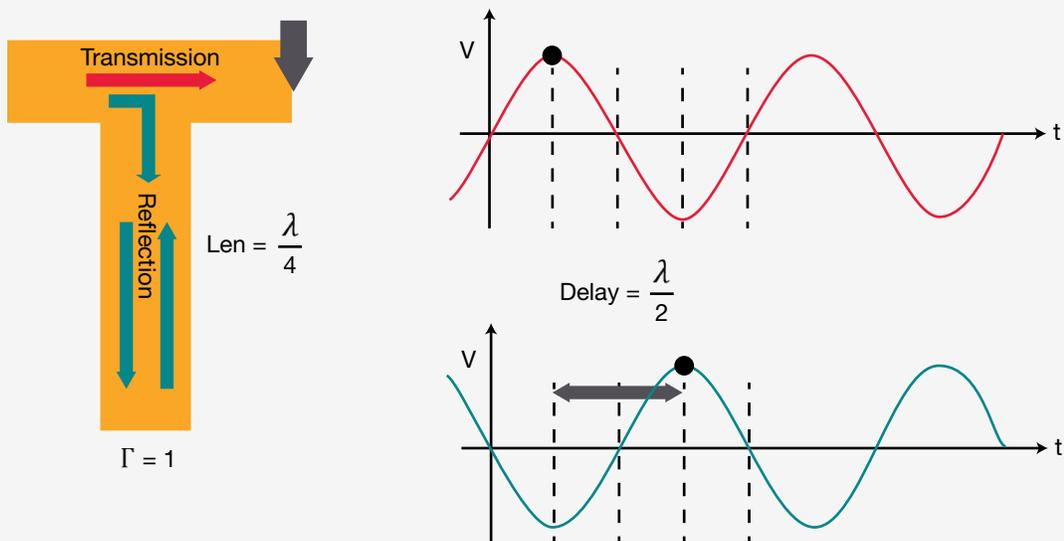
Figure 2: Effects of reflection on signal quality
