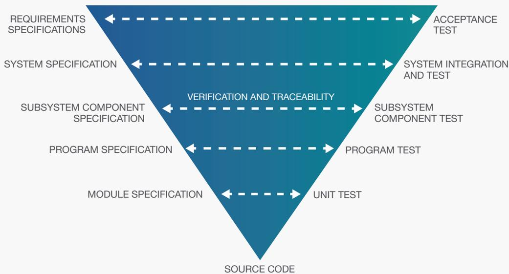
**Figure 3. The V development model maintains verification and traceability at all levels of the system.**
