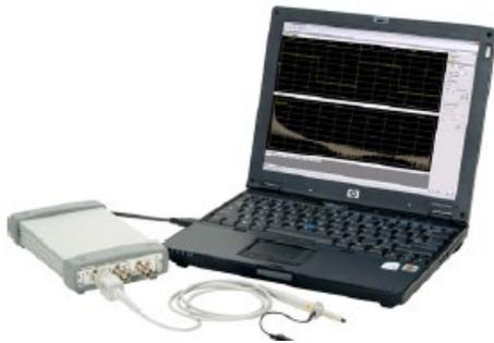
**Figure 1.** U2701/2A used as a standalone instrument
